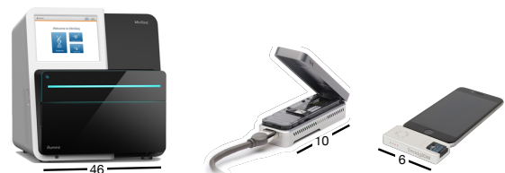
Figure 1: Illumina MiniSeq (left), vs. portable MinION (middle) and forthcoming SmidgION (right). Pictures not to scale. The approximate size in centimeters is marked for reference. The current price of MinION is $1,000 compared to $50K for an entry-level benchtop sequencer.
